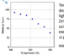
Temperature dependence of the light output of the ZnWO<sub>4</sub> crystal scintillator for excitation with <sup>241</sup>Am  $\alpha$  particles
