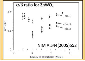
ZnWO<sub>4</sub> anisotropic scintillator: a very promising detector (NIMA544(2005)553, Eur. Phys. J. C 73 (2013) 2276): i) very good anisotropic features; ii) high level of radiopurity; iii) high light output, that is low energy threshold feasible; iv) high stability in the running conditions; v) sensitivity to small and large mass DM candidate particles; vi) detectors with ~ kg masses feasible
