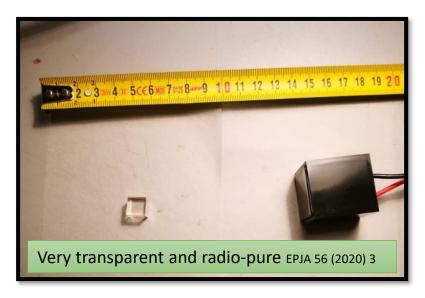
$ZnWO_4$  crystal = 10 x 10 x 10 mm<sup>3</sup> (detector of reduced dimensions to investigate neutron single-scattering)
