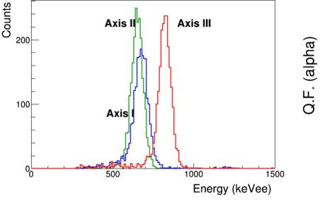
Energy spectra of 4.63 MeV  $\alpha$  particles impinging along the three axes of the crystal. The crystal was irradiated in the directions along the crystal axes I (blue on-line), II (green on-line), and III (red on-line), respectively
